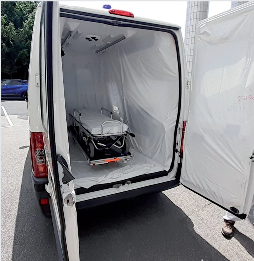
Figure 4: Transport vehicle, prepared with a vinyl coverage for transport of contaminated patients
